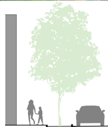
SECTION - TREE IN ROAD PROTUBERANCE
