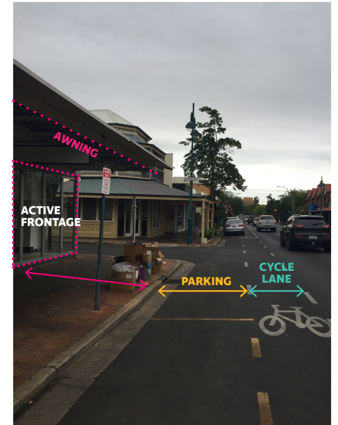
Melbourne Street East - Wide footpaths, activated frontages and awnings make for good walkability. Cycle lane bordered by parked cars on one side and traffic on the other creates an uncomfortable and unsafe environment for cyclists.
